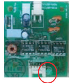
Indoor unit communication PCB
