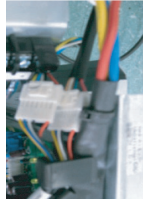
<Fan Motor Middle Connector>
