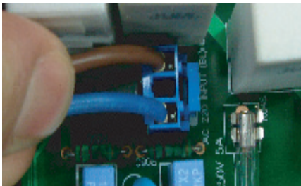
Inverter PCB assembly power connection
