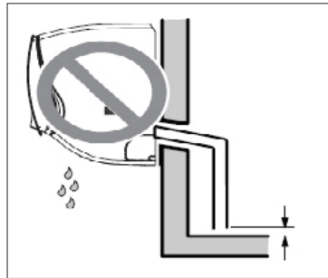
Case 8 : When the end of the drain hose abuts narrow the gap with the ground.
