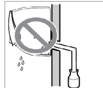
Case 3 : The end of the drain hose plugged into a bottle.
