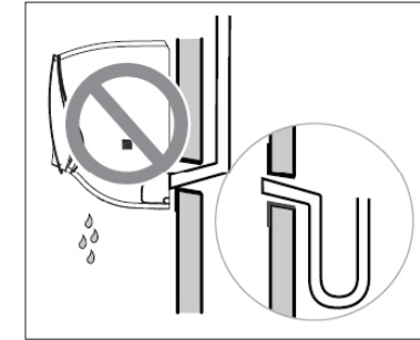
Case 2 : Installing without rain traps
