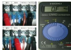
3) Check electric leakage Communication Line and Pipe
