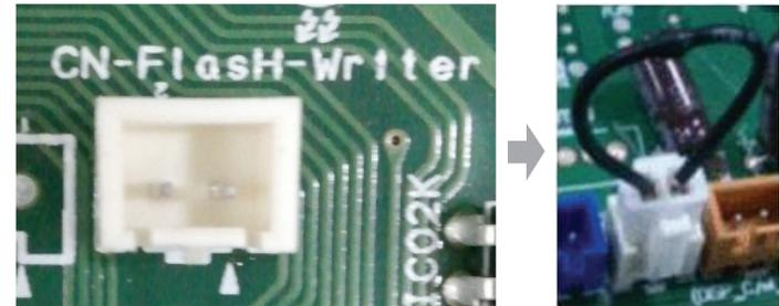
[Connector with capacitor in CN\_Flash\_Writer or CN\_Flash]
