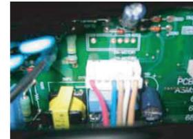
\*\* Replace the indoor unit PCB, and then make sure to do Auto addressing and input the address of central control
