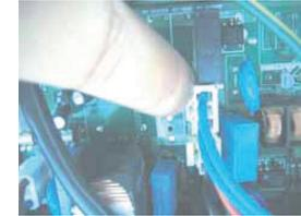
\*\*\* Indoor PCB drain pump connector
