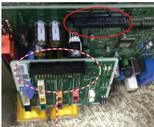
Ejection of sub PCB
