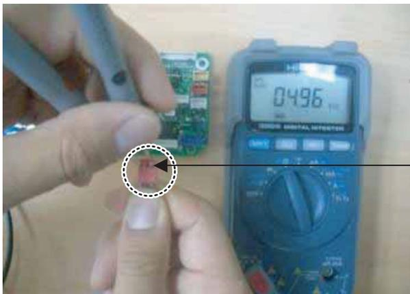
Measure the resistance of outlet pipe temp sensor.
