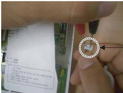
← Checking communication cable connection status
