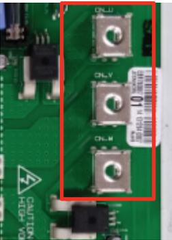
\* Check DC\_Link Connector joining condition
