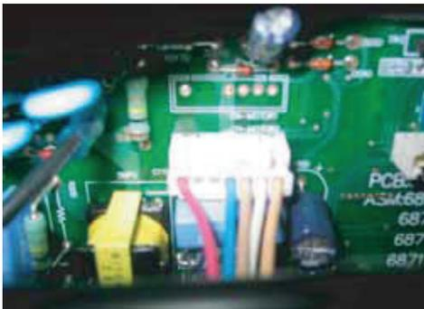
\*\* Replace the indoor unit PCB, and then make sure to do Auto addressing and input the address of central control
