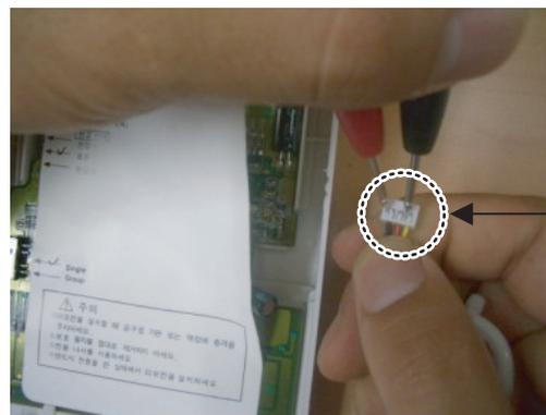
Checking communication cable connection status
