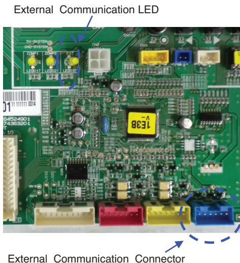
Communication Connector & LED in Main PCB
