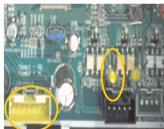
Communication Connector & LED in Comp2 PCB
