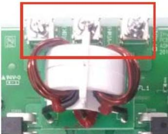
\* Check DC\_Link Connector joining condition
