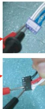
Check the resistance inverter compressor discharge temperature sensor
