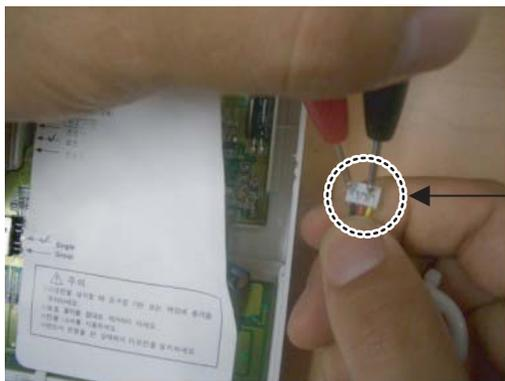
Checking communication cable connection status
