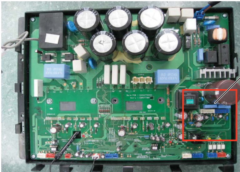
<FAN Motor Connection check>
