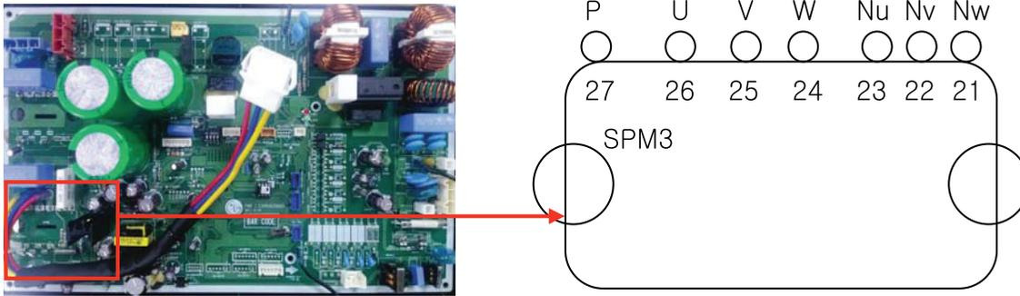
1. Wait until inverter PCB DC voltage is discharged after main power off.
