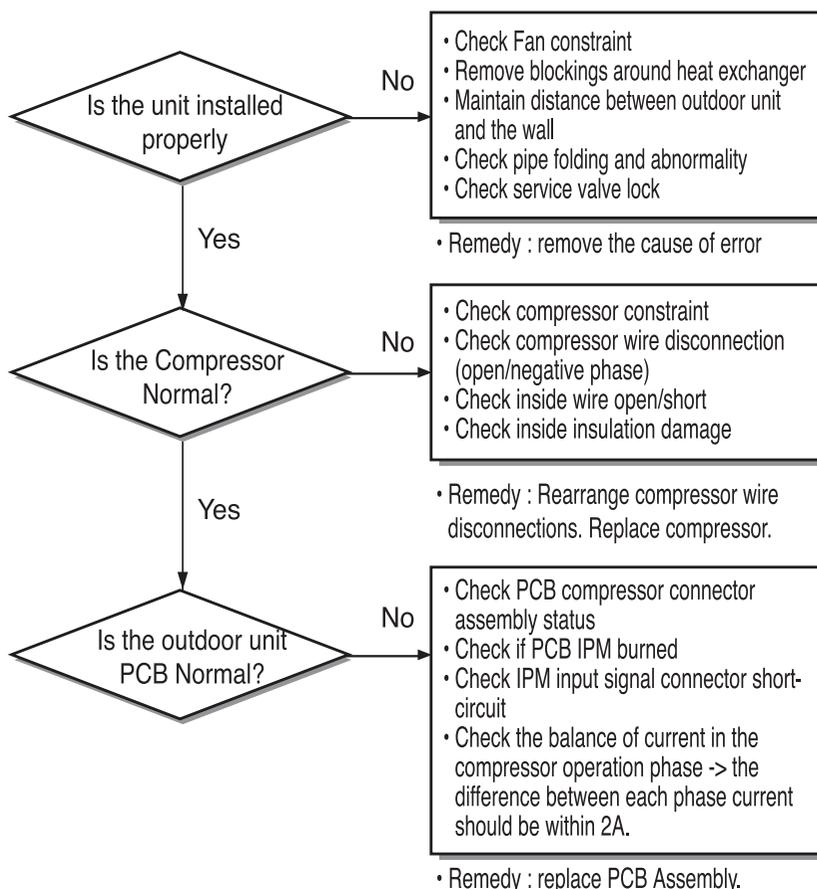
**• Check for short-circuit of PCB IPM Input Signal Connector.**
