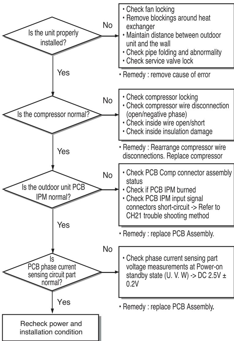
**Inspecting PCB phase current sensing circuit**
