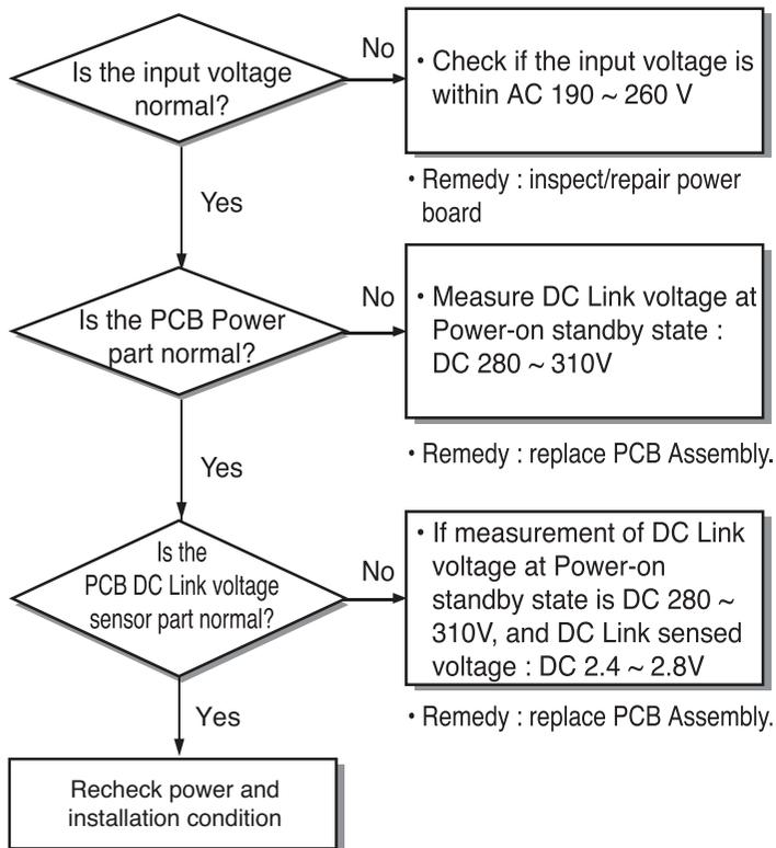
**• Inspecting PCB DC Link voltage sensing circuit**
