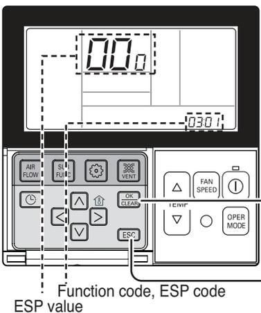
**6** Select ESP fan step again by using button and setup ESP value, as No. 4 and 5, that corresponds each wind flow
