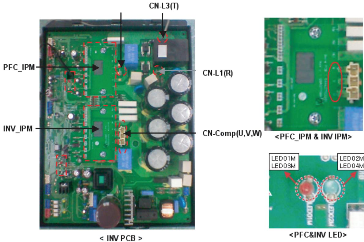
1. Wait until inverter PCB DC voltage is discharged after main power off.
