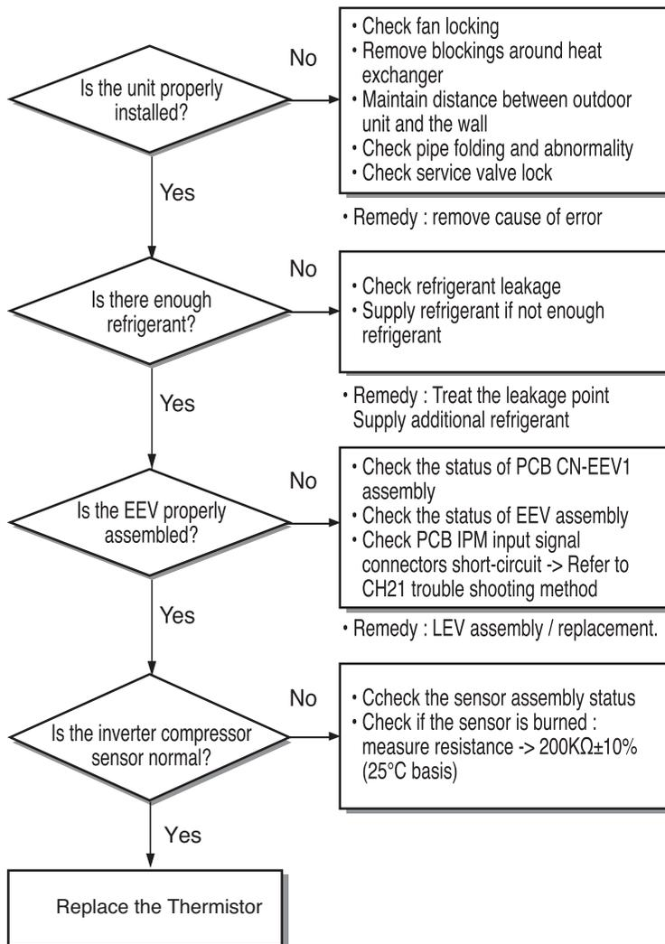
**Inspecting Inverter Compressor Discharge Sensor**
