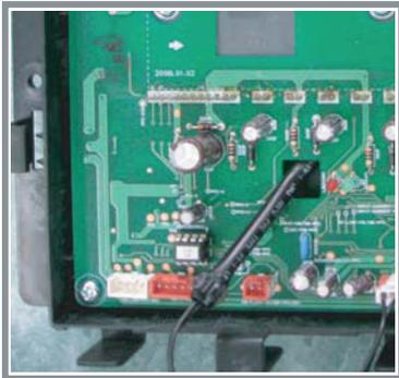
Comp frequency control according to heatsink temp.
