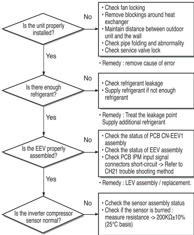
**• Inspecting Inverter Compressor Discharge Sensor**
