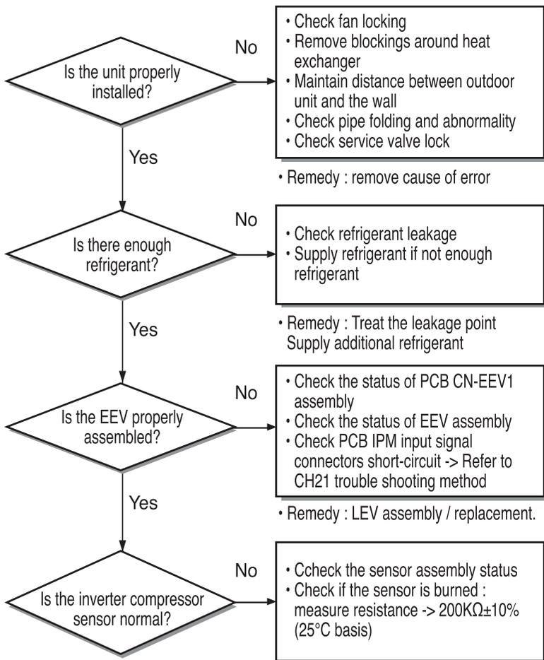
**Inspecting Inverter Compressor Discharge Sensor**
