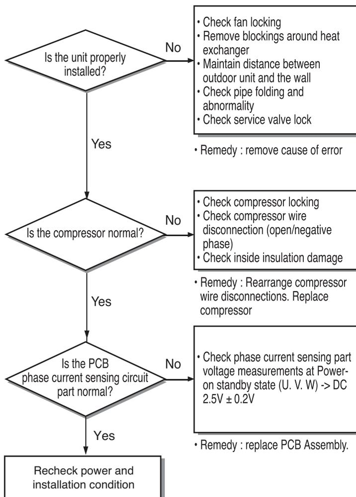
**Inspecting PCB phase current sensing circuit**
