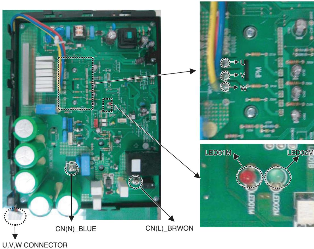
1. Wait until inverter PCB DC voltage is discharged after main power off.
