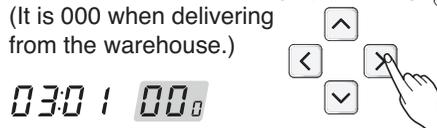
**5** Press button to setup ESP value.
