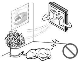
**Do not block the inlet or outlet of air flow.**
