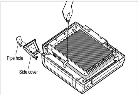
**NOTICE** When making pipe path through rear wall, you don't need to pick the pipe hole.
