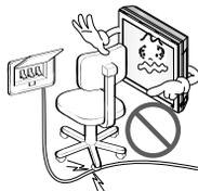
**Do not turn the air-conditioner ON or OFF by plugging or unplugging the power plug.**
