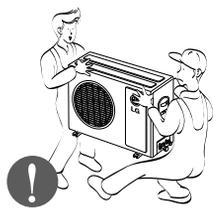
**Do not install the product where it will be exposed to sea wind (salt spray) directly.**
