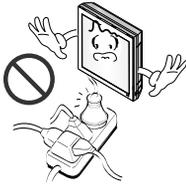
**Grasp the plug to remove the cord from the outlet. Do not touch it with wet hands.**
