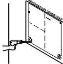
5. Drive the fore plastic anchors into drilled points.
